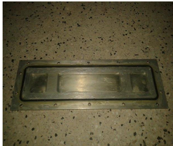
Fig. 7: O-ring in the lid of the electronics box
